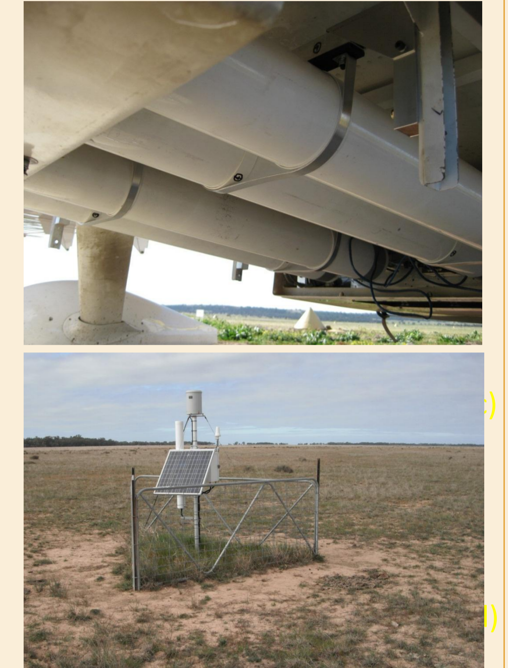
Fig. 2: (top) COSMOS Rover installed in the aircraft used for the surveys; (bottom) CosmOz tower in Yanco, Australia.
